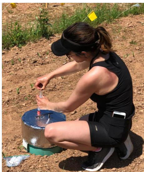
Sabrina Ellsworth, P.Ag., taking a greenhouse gas sample from a static chamber
